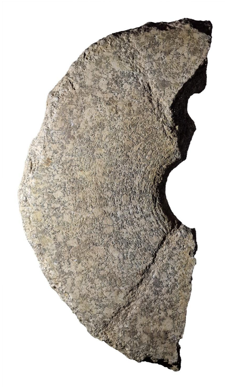
Fig. 3. Tresminas. Fragment of a catillus from an ore mill. The re-sharpening and concentric grooves on the grinding surface are clearly recognisable. Typically, the latter only formed towards the centre hole, while the actual grinding surface is smooth. (Foto Wahl-Clerici).
